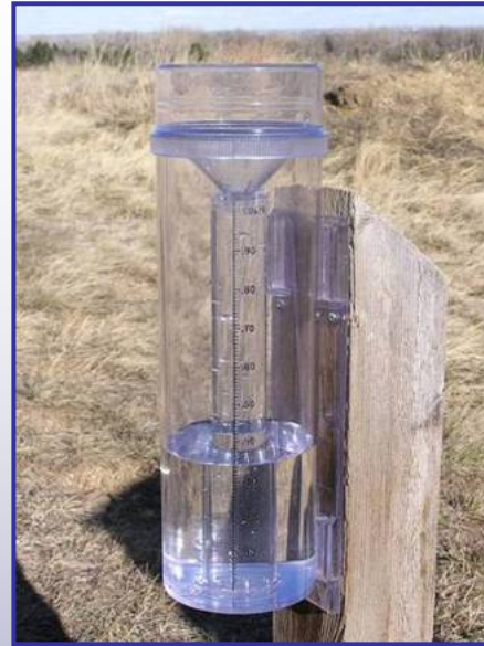
4-inch diameter high-capacity rain gauges
